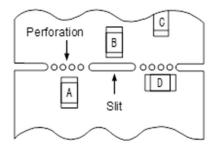
(3) Mounting components near screw holes
