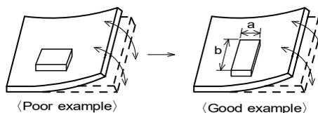
(2) Components location on PCB separation
