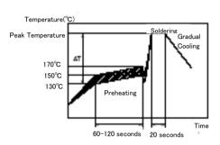
[Allowable Soldering Temperature and Time]
