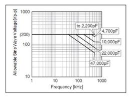
Chip(LxW): 2.0x1.25mm/3.2x1.6mm U2J(7U) Char. Rated Voltage:DC250V
