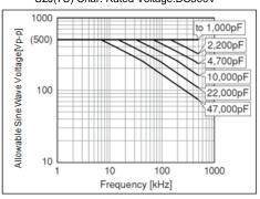
Chip(LxW): 3.2x1.6mm/3.2x2.5mm/ 4.5x3.2mm/5.7x5.0mm U2J(7U) Char. Rated Voltage:DC630V
