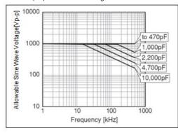
Chip(LxW): 3.2x1.6mm/3.2x2.5mm U2J(7U) Char. Rated Voltage:DC2 kV
