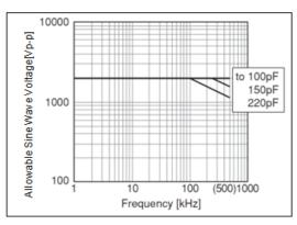
Chip(LxW): 4.5x2.0m U2J(7U) Char. Rated Voltage:DC3.15kV
