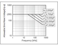
Chip(LxW): 3.2x1.6mm/3.2x2.5mm/ 4.5x3.2mm/5.7x5.0mm U2J(7U) Char. Rated Voltage:DC500V
