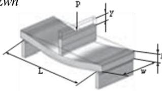
$\epsilon$  : Strain on center of board ( $\mu\text{st}$ )
