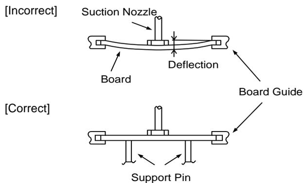
2. Dirt particles and dust accumulated between the suction nozzle and the cylinder inner wall prevent the nozzle from moving smoothly. This imposes greater force upon the chip during mounting, causing cracked chips. Also, the locating claw, when worn out, imposes uneven forces on the chip when positioning, causing cracked chips. The suction nozzle and the locating claw must be maintained, checked and replaced periodically.
