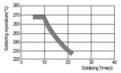
In the case of repeated soldering, the accumulated soldering time must be within the range shown above.
