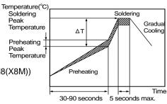
[Allowable Flow Soldering Temperature and Time]
