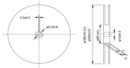
Fig.3 Taping Diagram
