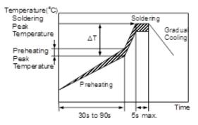
[Standard Conditions for Flow Soldering]
