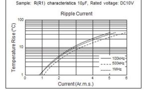
[Example of Temperature Rise (Heat Generation) in Chip
