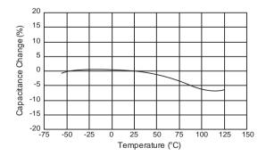
[Example of Temperature Characteristics X5R(R6)] Sample: 22µF, Rated Voltage 4VDC
