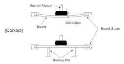
2. Dirt particles and dust accumulated between the suction nozzle and the cylinder inner wall prevent the nozzle from moving moving smoothly. This imposes greater force upon the chip during mounting, causing cracked chips. Also, the locating claw, when worn out, imposes uneven forces on the chip when positioning, causing cracked chips. The suction nozzle and the locating claw must be maintained, checked, and replaced periodically.
