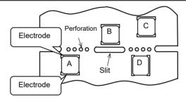
(3) Mounting components near screw holes
