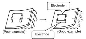
(2) Components location on PCB separation
