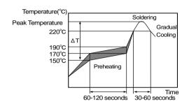
[Allowable Reflow Soldering Temperature and Time]
