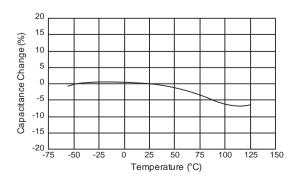
[Example of Temperature Characteristics R6] Sample: 22µF, Rated Voltage 4VDC
