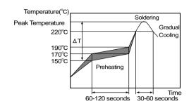
[Allowable Reflow Soldering Temperature and Time]
