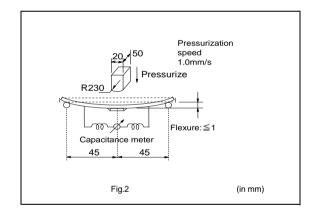
Adhesive Strength of Termination, Vibration Resistance, Temperature Cycle, Humidity, Humidity Load, High Temperature Load, Resistance to Soldering Heat (Reflow method)
