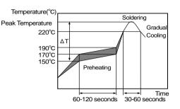
[Standard Conditions for Reflow Soldering]
