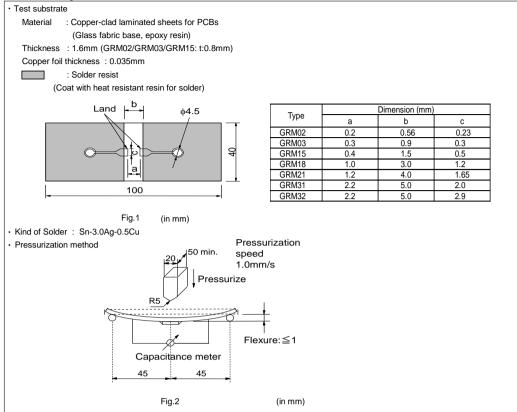
Adhesive Strength of Termination, Vibration, Temperature Sudden Change, Resistance to Soldering Heat (Reflow method)
