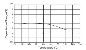
[Example of Temperature Characteristics X5R(R6)] Sample: 22μF, Rated Voltage 4VDC
